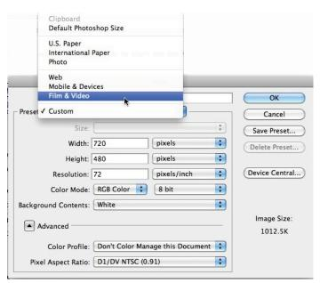
**2.** Next, click on Size to select your video's aspect ratio (dimensions). NTSC DV is for 4:3 (conventional TV dimension) and NTSC DV Widescreen is for 16:9 (modern flat panel TV dimension). Use one of the two "HDTV" settings for Blu-ray.
